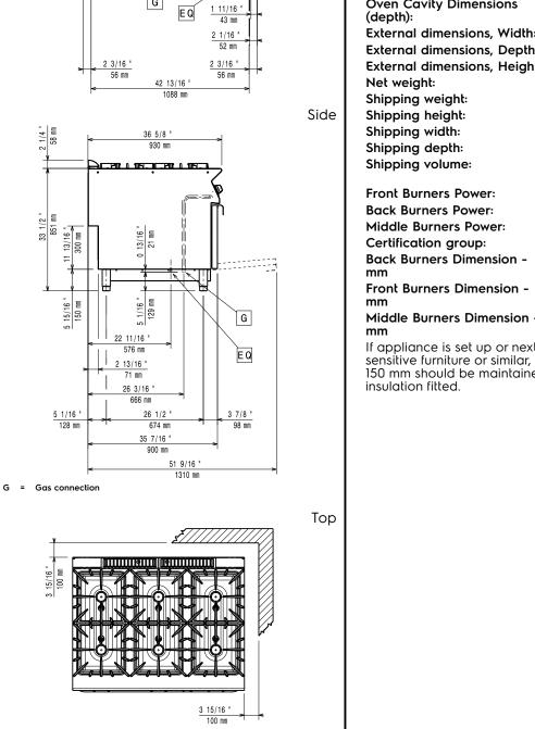
Modular Cooking Range Line 900XP 6-Burner Gas Range 10 kW on Large Gas Oven
